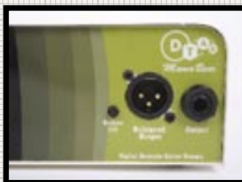
■ A low-impedance, balanced XLR out is best for hook-ups to a desk or recording console
